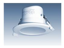
Powerful, completely encapsulated LED downlight 7 W, in robust plastic housing, with front glass and integrated power supply. Color temperature (CCT) adjustable by slide switch from coolwhite (approx. 6000 K), over neutralwhite (approx. 4000 K), to warmwhite (approx. 3000 K)
