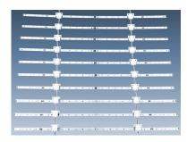
LED lattice light, IP66, for outdoor backlighting. Light consisting of 61 LED bars connected parallel in a distance of 30 mm. The single LED bar is fitted with 12 LEDs. Each bar 2.7 W and approx. 270 lm., dimensions 496 x 10 x 7 mm
