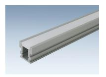
Walkable aluminium profile for floor mounting, with diffusor, with end caps. Suitable for led strips up to 11 mm width. Usuable in dry indoor areas
