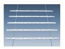
LED lattice light for backlighting large areas or displays. Light consisting of 27I LED bars connected parallel in a distance of 75 mm. Each LED bar is fitted with 6 high-power LEDs with front lens. Each bar 4.2 W and approx. 400 lm., dimensions 496 x 18 x 7 mm
