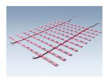
RGBW LED lattice light for coloured backlighting. Light consisting of 40 LED bars connected parallel in a distance of 30 mm. The single LED bar is fitted with 12 RGBW LEDs with front lens. Color temperature white 5000 K. Each bar 4.0 W (R-G-B-W each 1.0 W)., max. 197 lm (R: 26 lm, G: 65 lm, B: 16 lm, W: 90 lm), dimension 496 x 20 x 8 mm.
