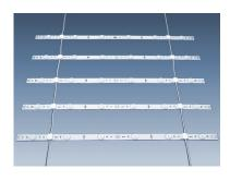
LED lattice light for outdoor backlighting, IP66 waterprotected by special varnish coating. Light consisting of 27 LED bars connected parallel in a distance of 75 mm. Each LED bar is fitted with 6 high-power LEDs with front lens. Each bar 4.2 W and approx. 400 lm., dimensions 496 x 18 x 7 mm
