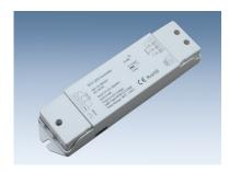
LED Controller for RGB-LED strips, bi-color strips (with adjustable color temperature; CCT adjustable) and for single color LED strips (or other LED lights). If connected to RGB strip/light max. 432 W (24 V) oder 216 W (12 V); Functions: color selection, dimming, several color changing programs If connect to single color LED strip/light max. 144 W (24 V) oder 72 W (12 V); Functions: Dimming. Remote needed. Multiple controllers can be grouped and controlled by one single remote
