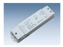
LED Controller for RGB-LED strips and for single color LED strips (or other LED lights). If connected to RGB strip/light max. 432 W (24 V) oder 216 W (12 V); Functions: color selection, dimming, several color changing programs If connect to single color LED strip/light max. 144 W (24 V) oder 72 W (12 V); Functions: Dimming. Remote needed. Multiple controllers can be grouped and controlled by one single remote
