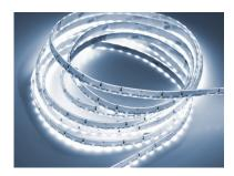
Flexible LED strip with side emitting LEDs, 14.4 W/m, 120 LEDs/m, width 8 mm, length 5 m (one reel), dimmable, every 5 cm cutable, self-adhesive
