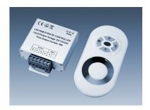
Controller for RGB LED strips and lights, with remote control. Functions: Smooth color selection, dimming, preprogrammed color change, on/off switching. For max load of 144 W (24 V). Up to 10 controllers can be controlled synchronously by one single remote control
