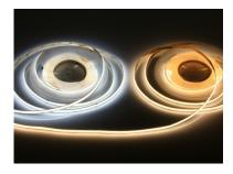
Dot-free flexible COB LED strip (608 chips/m) with adjustable color temperature from warmwhite to coolwhite (approx. 2700 K to 6500 K), creating an uniform light band without any visible LED dots (totally dot-free), beam angle 180°, CRI > 90, self-adhesive, width 10 mm, dimmable, length 5 m, cuttable each 26 mm
