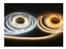
Dot-fee flexible COB LED strip (608 chips/m) with adjustable color temperature from warmwhite to coolwhite (approx. 2700 K to 6500 K), creating an uniform light band without any visible LED dots (totally dot-free), beam angle 180°, CRI > 90, self-adhesive, width 10 mm, dimmable, length 5 m, cuttable each 26 mm
