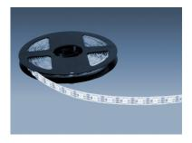
Flexible LED strip, equipped with individually addressable RGB LEDs, 18 W/m max., 60 LEDs/m, width 10 mm, length 5 m (one reel), dimmable, cutable at each LED, self-adhesive. Addressable with controller with pre-programmed special effects (e.g. LED flow lights), or with completely freely programmable controllers for individual special effects. Power supply by transformer 5 V DC
