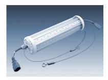
LED light for backlighting three-dimensional forms, like picture cubes and light pillars. Equipped with 96 LEDs, covered by protective glass. With suspension system for easy installation. Power supply by 100-240 V, no external driver needed. Max. 6 lights can be daisy-chained.
